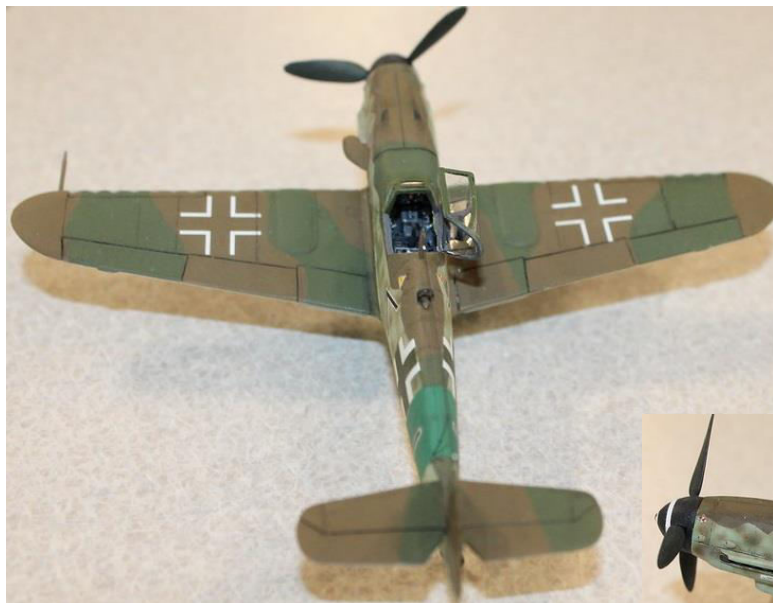
John Walker presented his 1/72nd scale Airfix BF109 K4 for review. He added multiple details to the model. He also removed and re-scribed panel lines. The plane was painted with Vallejo paints.
